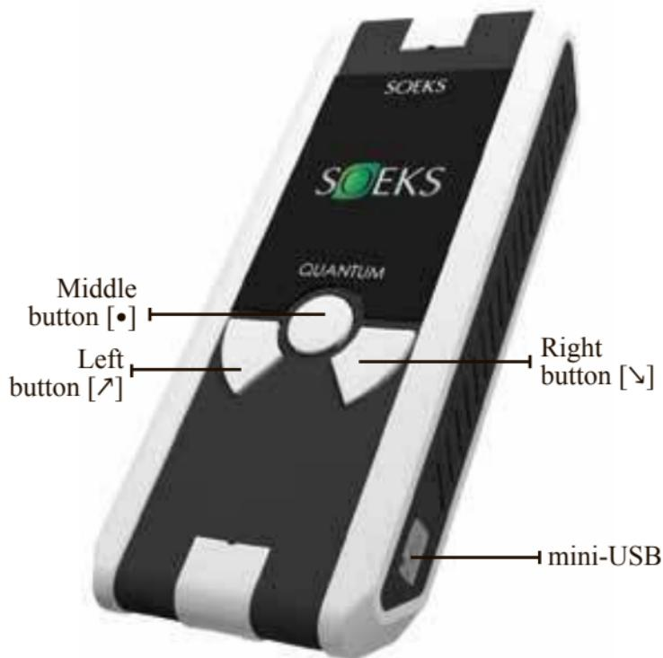
Left button [↗] - scrolls the menu (list) up. When the top (first) position on the list is reached, the cursor moves to the bottom (last) position. Decreases the value of the parameter.
