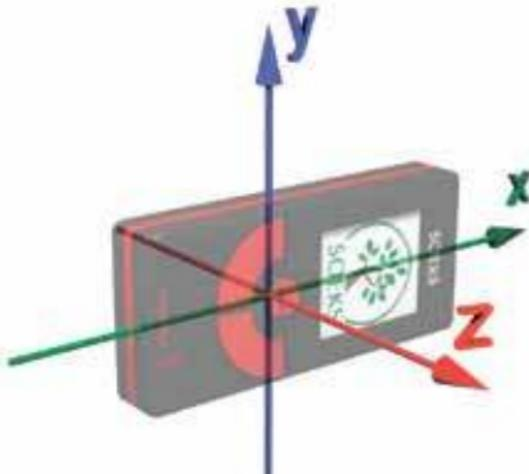
During the source search it is essential to analyze the instant values along individual axes for the purpose of source direction identification.
